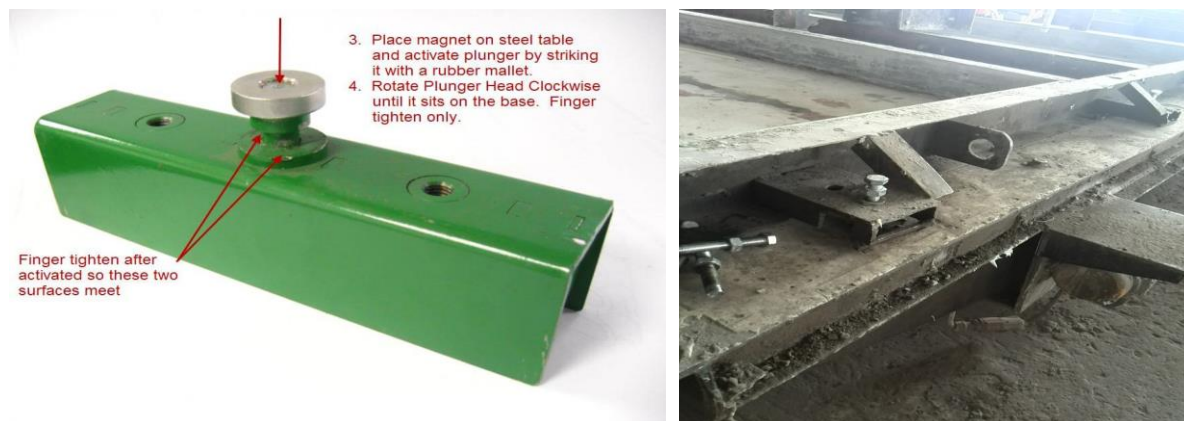
Fig 3.3 Illustrating magnet locking in contrast to the nut bolt system used presently
